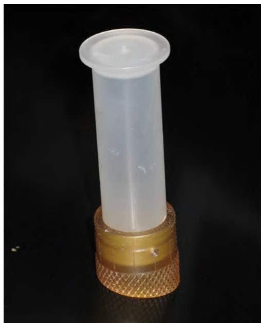
Fig. 2. Recording chamber and plastic cylinder. The cylinder must fit snugly within the recording chamber so that the long axis of the cylinder is parallel to the long axis of the cylinder.
